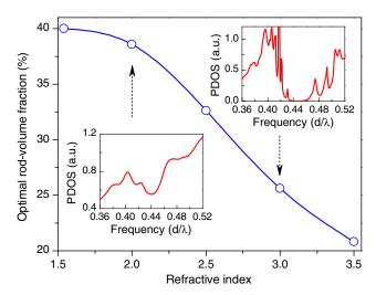
**Fig. 4.** Calculated optimal rod-volume fraction of RAD-PCs as a function of the refractive index of the rods. *Insets* show the PDOS for two cases: one with a photonic pseudogap at refractive index n=2, and the other with a complete photonic bandgap at n=3. The threshold for a complete photonic bandgap in these amorphous structures is  $n \sim 2.3$ .
