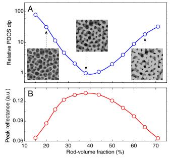
**Fig. 3.** (A) Calculated relative PDOS dip for the model RAD-PC for different rod-volume fractions. *Insets* are cross-sectional images of the model RAD-PC with volume fractions of 20%, 38%, and 65%. (B) Calculated peak reflectance for the RAD-PC slab with various volume fractions. Circles are calculated data, and the lines are a guide to the eye.
