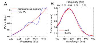
**Fig. 2.** (*A*) Calculated PDOS for the model RAD-PC as a function of reduced frequency  $d/\lambda$ , where d is the rod length and  $\lambda$  is the vacuum wavelength. The PDOS for a homogeneous medium with refractive index n=1.23, a volume-weighted average, is also given for comparison. (*B*) Normalized calculated and measured reflection spectra under normal incidence. The calculations were based on observed d=170 nm.
