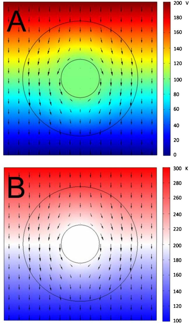
FIG. 3. (Color online) Finite element simulations of the cross section of our designed cloak with  $R_1:R_2=1:3$ . Parameters are set to be 300 K and 200 V at the top boundary and 100 K and 0 V at the bottom boundary. (a) The arrows display the pathway of the current density in the cloaking shell; color surface represents the electric potential. (b) Here arrows denote the pathway of heat flux in the cloaking shell and the temperature distribution is indicated by the color surface.
