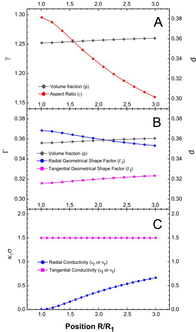
FIG. 4. (Color online) The calculation results for a cloak with  $R_1:R_2=1:3$ . (a) The shape aspect ratio and volume fraction of the nonspherical nanoparticles as functions of position (indicated by  $R/R_1$ ). (b) The radial and tangential part of geometrical shape factors as functions of  $R/R_1$ . (c) The normalized values of the effective electrical and thermal conductivities at different positions in the cloak shell with  $R_1:R_2=1:3$ .
