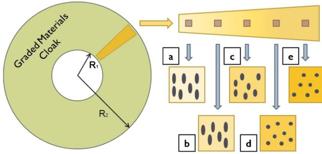
FIG. 1. (Color online) Schematic diagram of our designed cloak.  $R_1$  and  $R_2$  are the radii of the inner and outer boundaries of the cloaking shell, respectively. The nonspherical nanoparticles are distributed along the radius of the cloak with various shape aspects and volume fractions.
