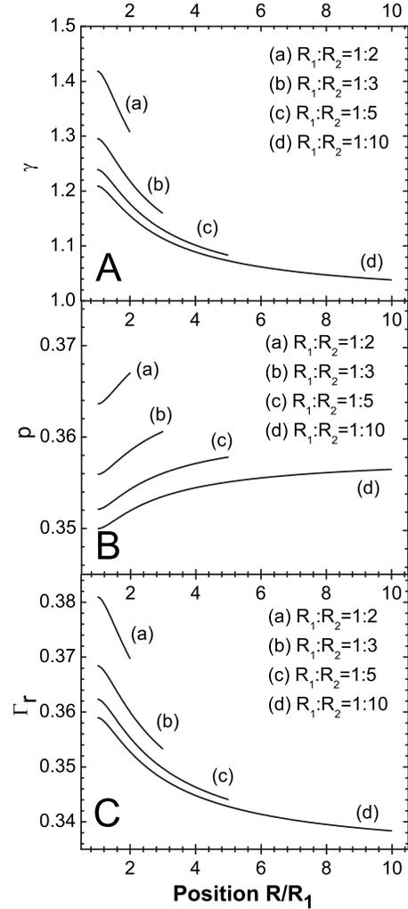
FIG. 5. Comparison of the parameters for different cloaks with  $R_1:R_2=1:2, 1:3, 1:5$ , and  $1:10$ . (a) The shape aspect ratio  $\gamma$  of nonspherical nanoparticles, (b) the volume fraction  $p$ , and (c) the radial geometrical shape factor.
